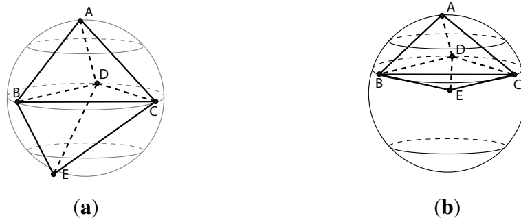
Figure 4. Illustration of a Delaunay unit tetrahedron cell (DUTC), under an arbitrary (non-unit disk graph (UDG)) communication model. (a) DUTC; (b) non-DUTC.
