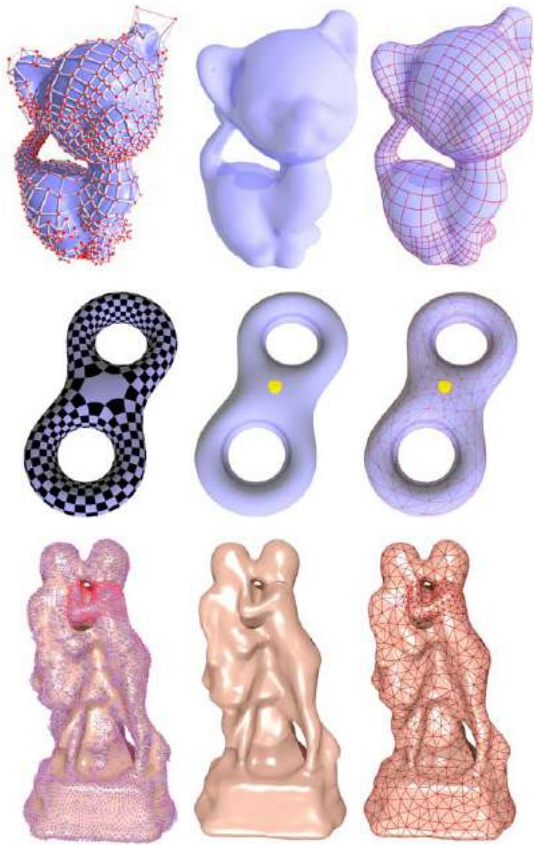
Fig. 8. Manifold splines are used to verify the theoretical results. These spline surfaces are of C^2 continuous, thus, the principal curvatures, normals, Hausdorff distance, etc, can be obtained analytically.
